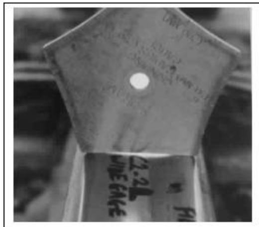
Figure 8. Shows a 12 inch (300mm) radius gage on the low rail and the damage caused by the false flange. Grinding of wide gage track must remove a substantial amount of metal from the field side to protect the rail from wheel false flange damage.
