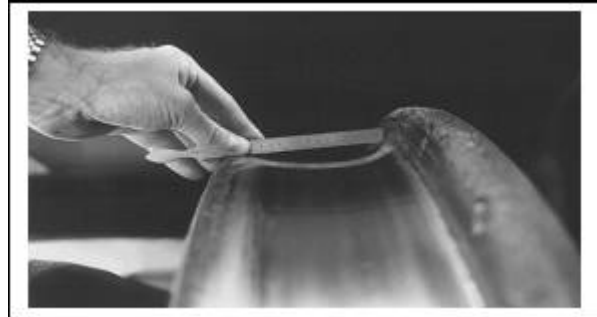
Figure 7. The rim side of the wheel may have a "false flange" which can cause significant damage to the low rail of sharp curves
