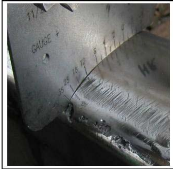
Figure 6. High rail gauge face shelling between 40 and 60 degrees, shown on the template, which is caused by lower natural wear and high lateral forces in curves with 100% effective gauge face lubrication.
