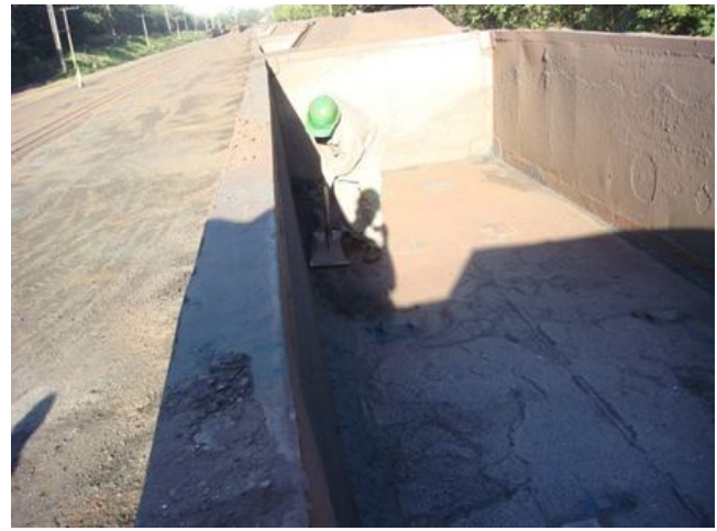
Figure 2. Manual wagon cleaning – using shovels
